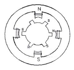
Fig. 1 Stepper motor-Four pole structure
