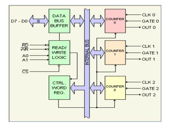
**Block Diagram of 8253-Programmable Interval Timer**
