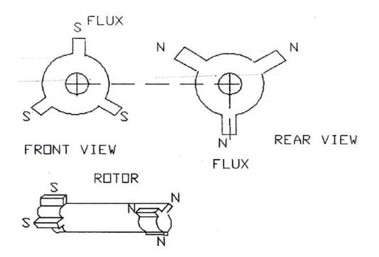
Fig. 2 Stepper motor- Cross sectional view
