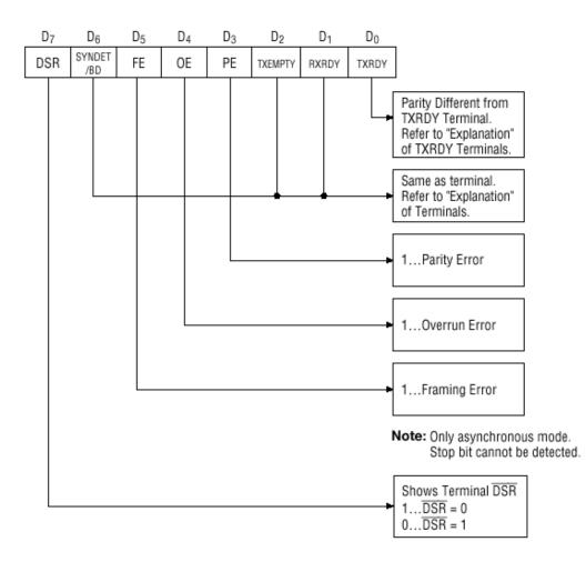
Fig. 7: Bit Configuration of Status Word
