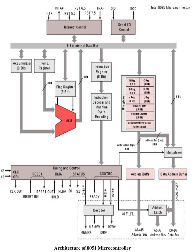
Architecture details of 8085 Microprocessor
