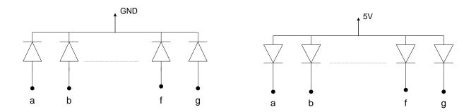
For a common anode display, a low is applied to a segment to turn it on. For a Common cathode display a high is applied to a segment to turn it on. In this board Common cathode display is used.
